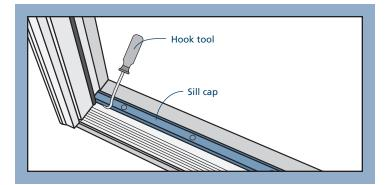
2. Pull up and out to disengage the sill cap and work your way down the threshold to remove completely.
